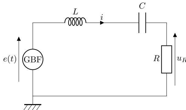
$$e(t) = E_m \cos(\omega t) \quad \rightarrow \quad \underline{e}(t) = E_m e^{j\omega t}$$
